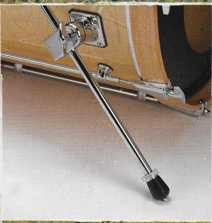
Surface mounted bass drum spurs offer maximum stability without interfering with the natural tone. Die-cast bracket, steel rods with rubber feet or optional floor gripping spikes are adjusted by a single wingnut that simultaneously clamps two jaws around the solid rod and sets the forward rake, height and level of the spur.
