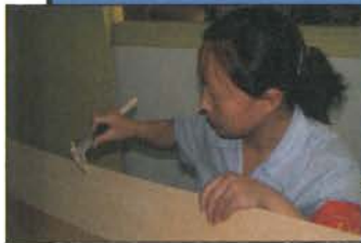
Veneers of maple, cherry, mahogany, and other woods are trimmed to exact sizes prior to being molded into drumshells.
