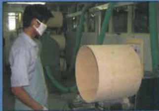
After the shells have been formed, they receive their bearing edges.
