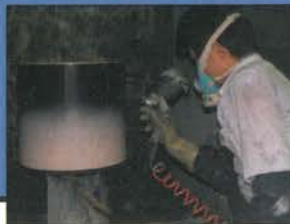
Every shell is carefully sanded, inside and out.
