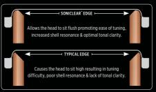
The SONIClear™ Bearing Edge implemented on the 30th anniversary snare drum allows the drumhead to sit flatter and make better contact with the shell. The result is a clearer fundamental pitch, effortless and consistent tuning, and a significantly expanded tuning range.
